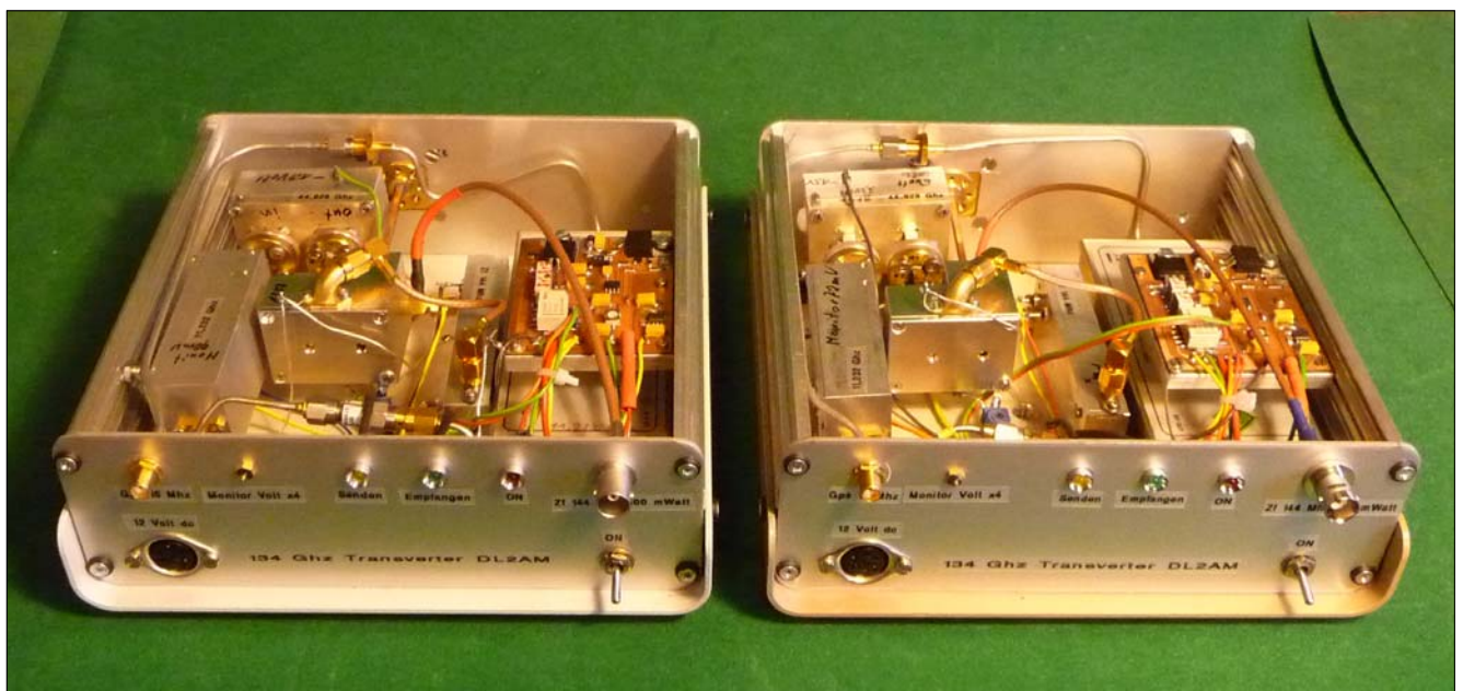
Fig. 7: Two 134 GHz transverters – ready for 2-way QSOs
